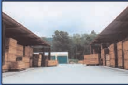
Lumber stored under T-sheds.
